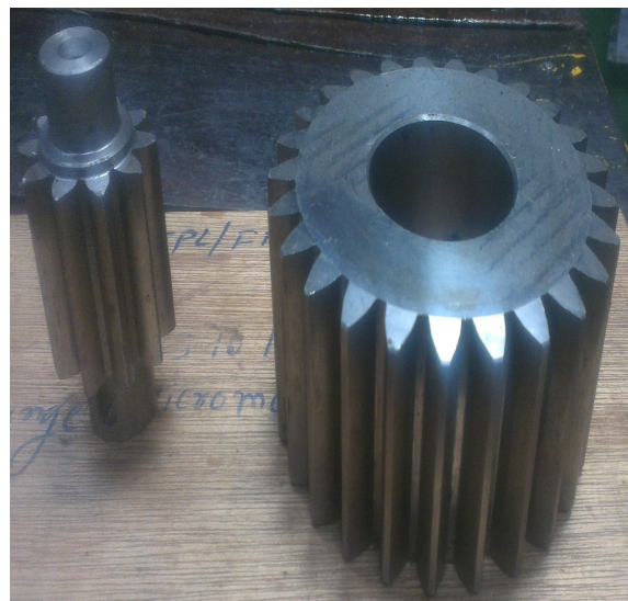
Figure 3. Spur gear produced by CNC gear hobbing machine
